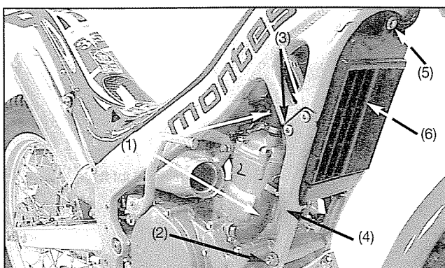
(1) WATER HOSES (2) HANGER BOLT (3) DOWN TUBE BOLTS (4) DOWN TUBE (5) BOLT (6) RADIATOR
